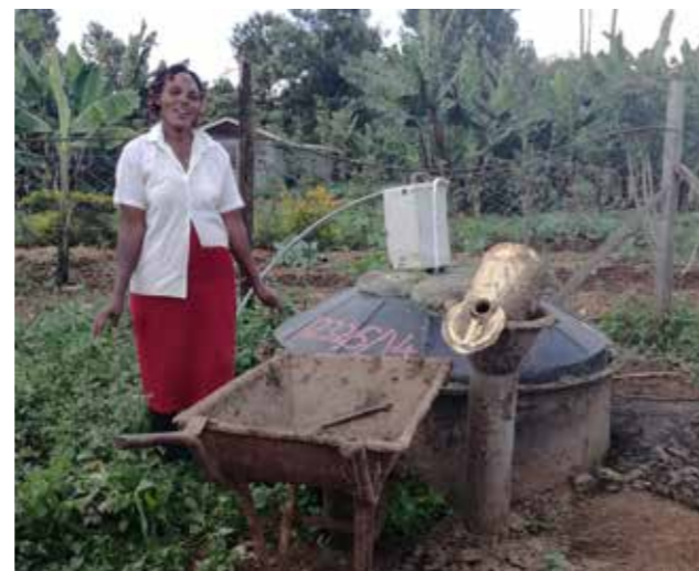
Grace Njatha feeding her floating drum biogas digester at her Githunguri farm in Kiambu
